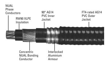
\*Single conductor armoured cables should not be used in hazardous locations. The armour and concentric bonding conductors of single conductor metal sheathed and metal armoured cables may carry a standing voltage with respect to ground, which is directly proportional to the magnitude of the current in the conductor, and the length of the cable, which may create sparks if grounded.
