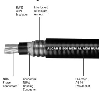
\*Single conductor armoured cables should not be used in hazardous locations. The armour and concentric bonding conductors of single conductor metal sheathed and metal armoured cables may carry a standing voltage with respect to ground, which is directly proportional to the magnitude of the current in the conductor, and the length of the cable, which may create sparks if grounded.
